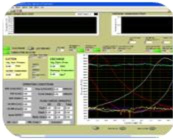
Quantum Controls, Inc. had the challenge of designing a gas compressor data acquisition system capable of synchronizing samples from multiple sensors to the rotational position of the pistons' crankshaft and performing measurements from field mounted meters and thermocouples.
