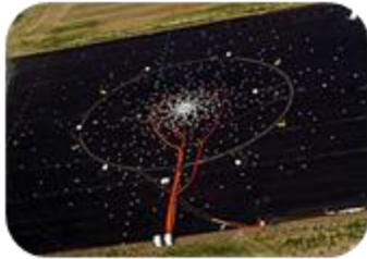
As part of the Quiet Technology Demonstrator 2 (QTD2) project, Boeing flight tested new technologies intended to reduce noise generated by its aircraft. Measuring the improvement these technologies provide required a flexible, accurate, and scalable test system to perform phased array acoustic imaging during the tests. They needed a distributed system architecture with the ability to expand to up to 1,000 channels or more while still maintaining tight timing and synchronization between channels.
